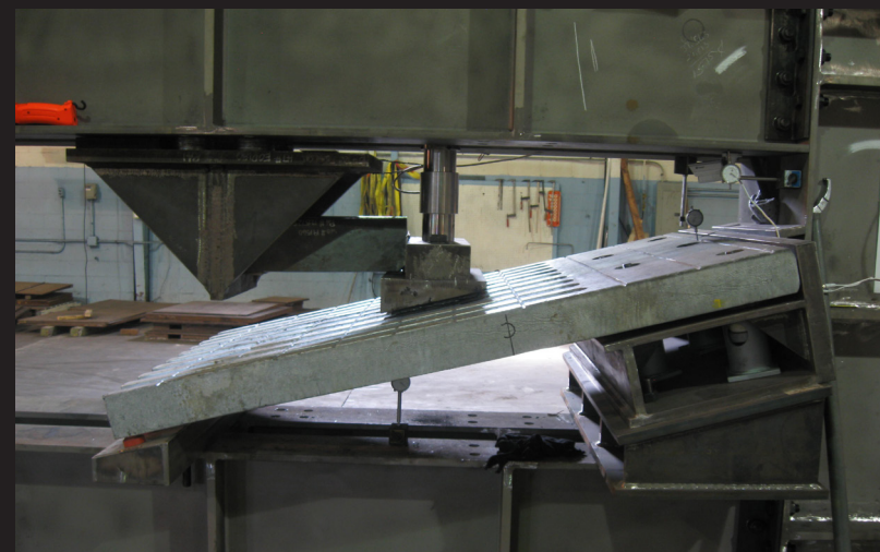
Fatigue Test on a Large Displacement Finger Joint
