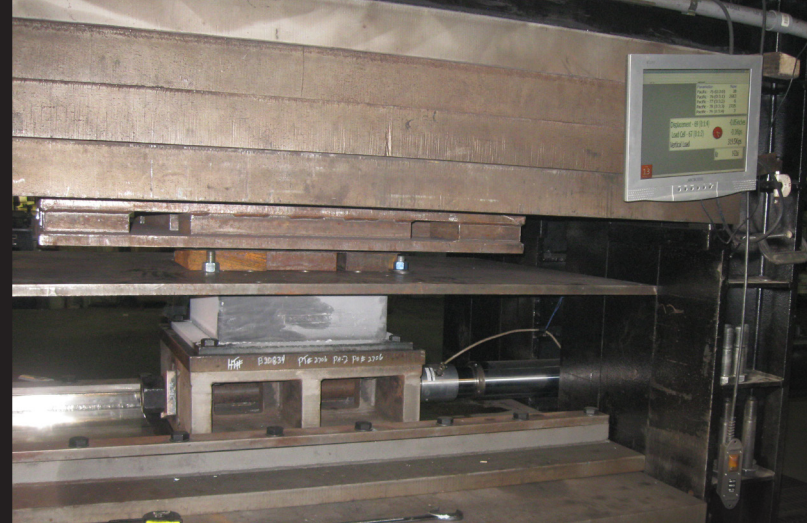
Cryogenic (-25C) Horizontal Stiffness Test on an Elastomeric Bridge Bearing. 10 inch displacement, using RJ Watson's 48 inch Actuator
